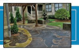
Exterior Kolour Dye™ is a translucent, UV stable dye, formulated using color designed to penetrate exterior and interior cementitious surfaces. Exterior Kolour Dye™ creates a unique. multi-colored translucent color scheme that unlike paints, will not crack, chip, or peel. Exterior Kolour Dye™ can be combined to create an unlimited color palate that creates a beautiful marble effect, when used properly. Create the look of a beautiful, custom acid stained floor in about 1/3 of the time.
